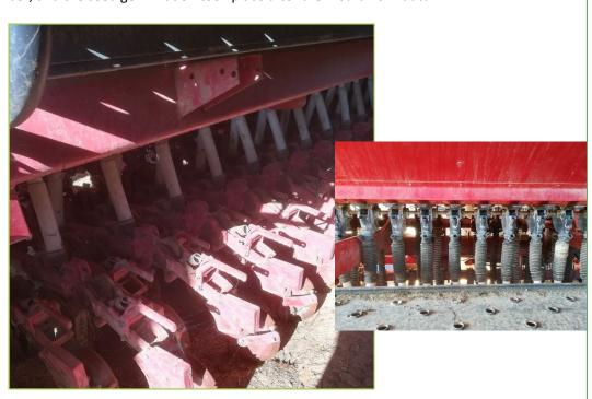
The sod-seeder used by the farmers (Semeato, mod. TDNG 520 SEED) has been designed for small grains and weights 9 tons. It is equipped with a seed box that can contain 2000 kg of seeds. The number of rows seeded is  $32 \times 17$  cm (7 m width).
