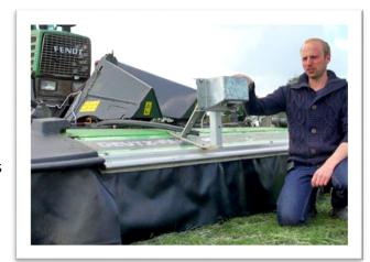
use of light reflection, the density and the dry matter content of the grass are determined.
